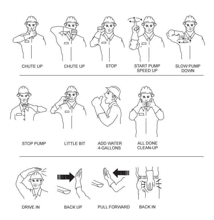
Figure 6. Operation Hand Signals
